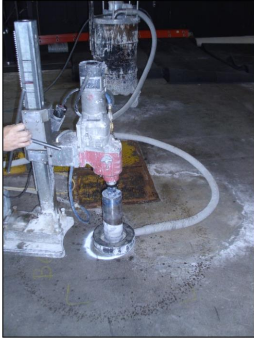
Concrete Coring Within the Former Auto Shop (Adjacent to a Former Vehicle Hydraulic Lift)
